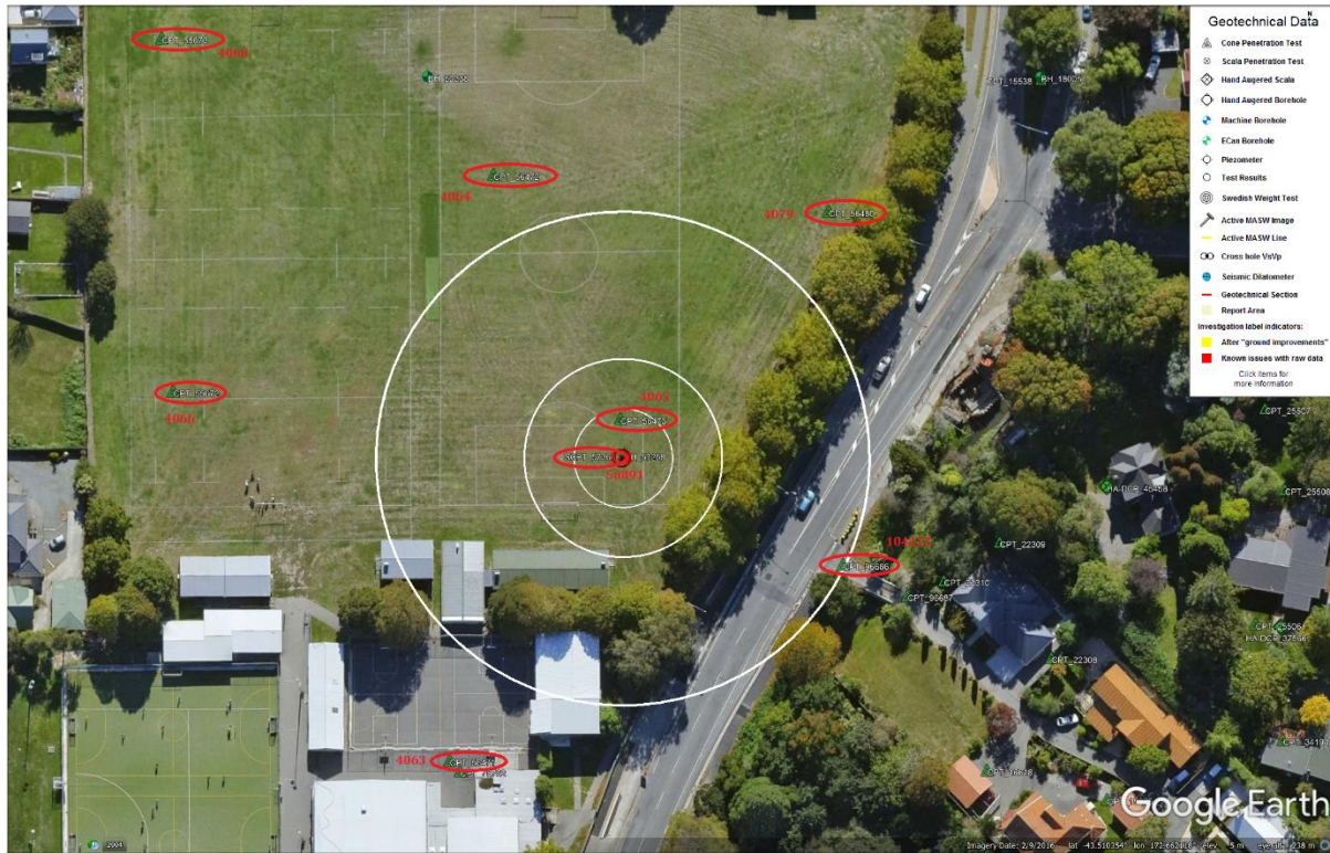
Figure 64. Locations of Cone Penetration Tests (CPTs).
